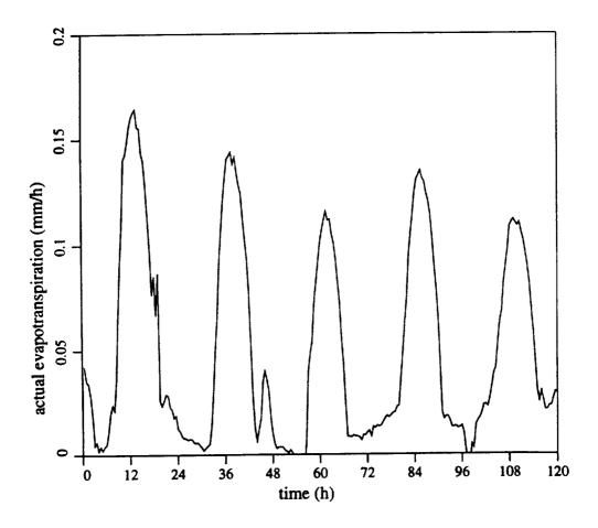
Figure 4. Evapotranspiration computed for the King's Creek catchment during FIFE IFC4, October 5-9, 1987 (control run). Time 0 corresponds to 445 GMT, October 5.
