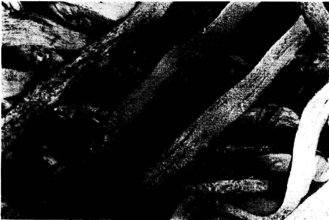
Figure 3. Photomicrograph of 90° cross-sectional view of a uniform construction showing cracking in tows found in pretest specimens.
