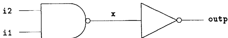
Figure 4: Implementation of an AND-gate from an NAND-gate and an inverter.
