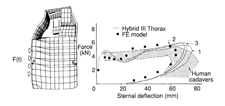
Figure 3. ATD thoracic response for pendulum impact (Ref. 2).
