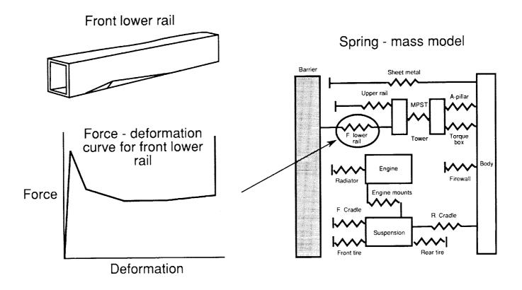
Figure 10. Optimum design with crashworthiness constraints (Ref. 5).
