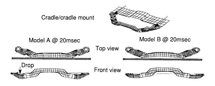
Figure 5. Two detailed models of an engine cradle (Ref. 3).
