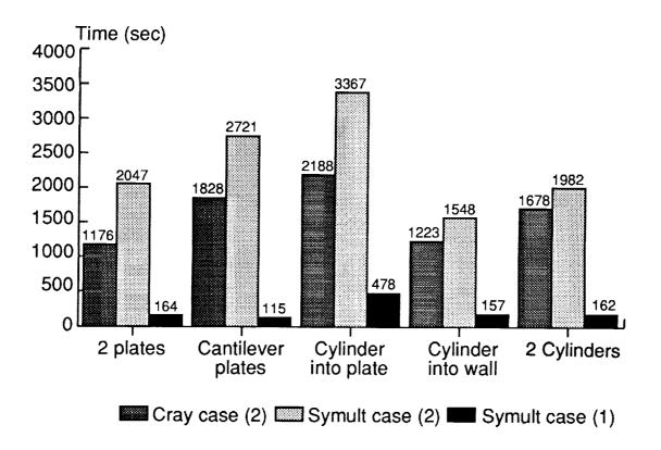
Figure 8. Comparison of execution times for case(1) (improved parallel contact) and case (2) (no parallel contact) (Ref. 4).
