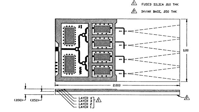
Figure 3. Initial 30 GHz phased array module design showing cavities and the integral radiating elements.
