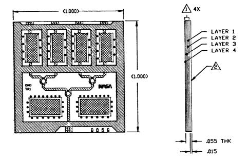
Figure 2. Initial 30 GHz mulitchip module design showing cavities for the two ASICs and four MMIC phase shifters.
