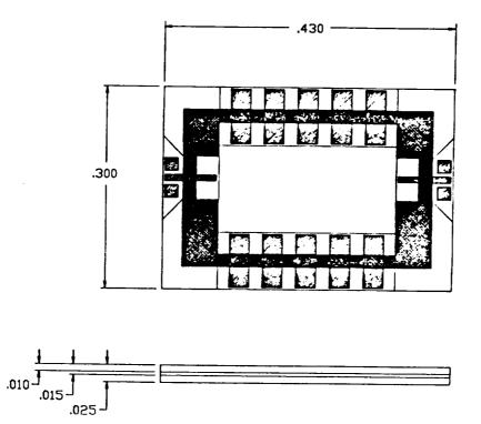
Figure 1. Initial DC to 30 GHz package design with two RF feedthroughs and 10 DC I/Os.
