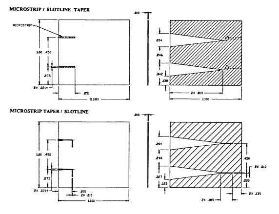
Figure 14. Two possible designs for the Task 3 radiating elements.
