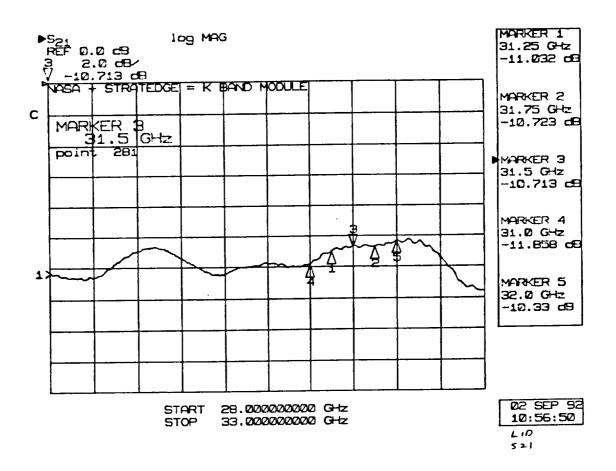
Figure 11. Plot of Wilkinson Power Divider insertion loss from port 1 to port 2 with the lid.
