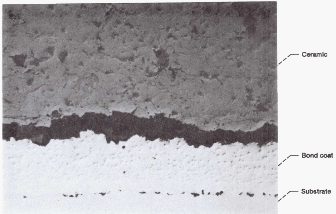
Hot zone after failure
