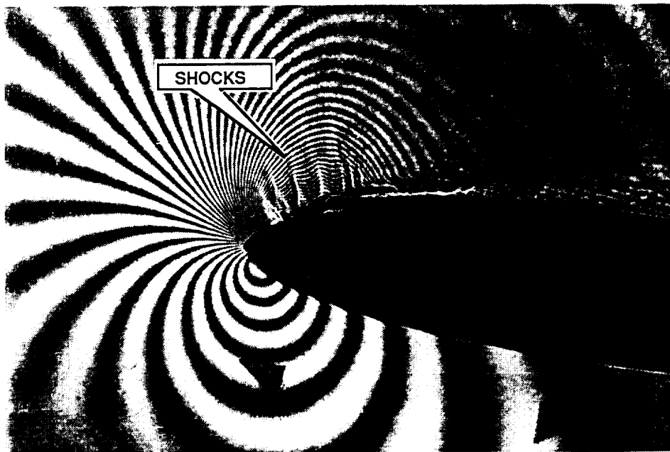
Fig. 7. Multiple Shocks on a Rapidly Pitching Airfoil: M = 0.45 , \alpha^+ = 0.0313 , \alpha = 12.6^\circ .
