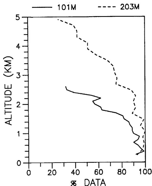
Figure 1. Percent of time wind data were successfully collected by the UHF wind profiler at 101-m (solid line) and 203-m (dashed line) resolutions.
