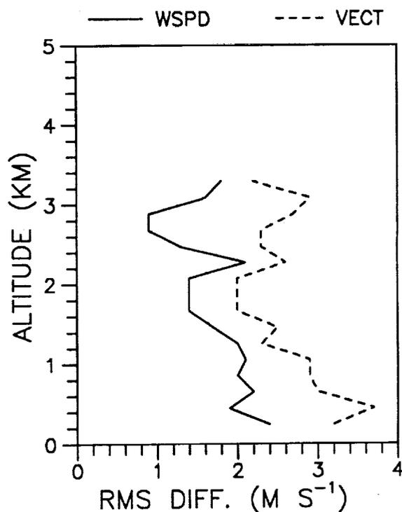
Figure 2. Rms wind speed differences (solid line) and vector wind differences (dashed line) of concurrent UHF wind profiler and rawinsonde data.
