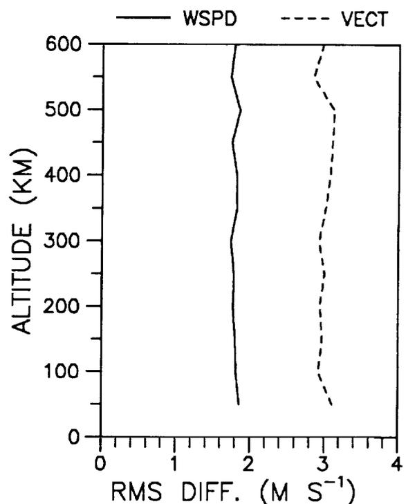
Figure 4. Rms wind speed differences (solid line) and vector wind differences (dashed line) of concurrent A0 and PA2 sodar wind data.
