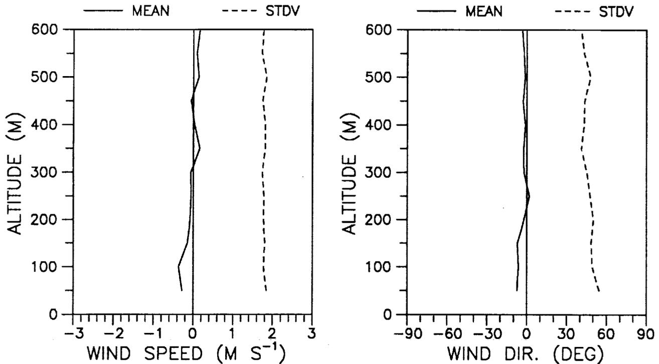
Figure 5. Means (solid lines) and standard deviations (dashed lines) of the differences in concurrent A0 and PA2 sodar wind speeds and directions.
