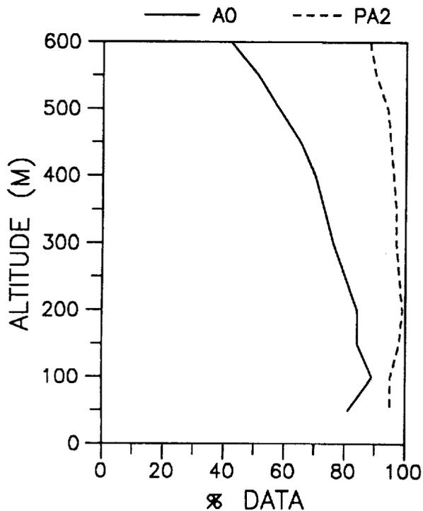
Figure 3. Percent of time horizontal wind data were successfully collected by the A0 (solid line) and PA2 (dashed line) sodar.
