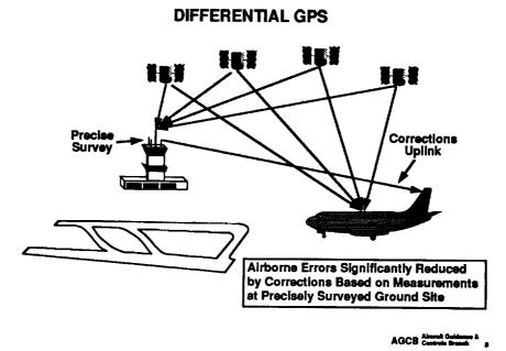
This viewgraph depicts the basic concept of differential GPS. The basic concept is to improve the airborne navigation solution by transmitting corrections to the airborne system based on GPS measurements made at a fixed site whose position is precisely known. The fixed ground site makes measurements of the satellites in view and computes corrections to the measurements based on its known location. These corrections are then transmitted to the airborne system (or ship, train, etc.) and processed
