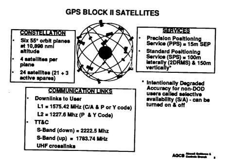
The GPS satellites will be contained in six 55° orbital planes 10,898 nautical miles above the earth which results in 12-hour orbits. Four satellites will be in each plane for a total of 24 satellites. Twenty-one of the satellites will be active and 3 will be spares for use in the advent of a satellite malfunction or failure.
