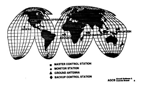
This viewgraph shows the location of the various ground stations and equipment for the GPS Control Segment. The master control station is located in Colorado Springs with a backup control station located in California. Monitor stations are located in Hawaii, Ascension Island, Diego Garcia, and Kwajalein.
