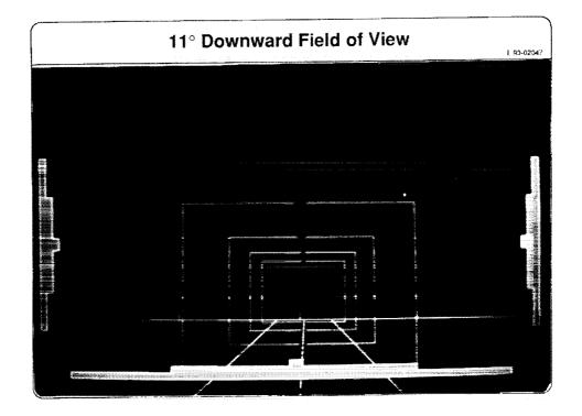
This slide illustrates the view for the default value of 11° for the downward field of view. The picture was taken on an ascending straight path. The fact that the HITS path is ascending can be ascertained by the fact that the vanishing point of the lane stripes is above the horizon.
