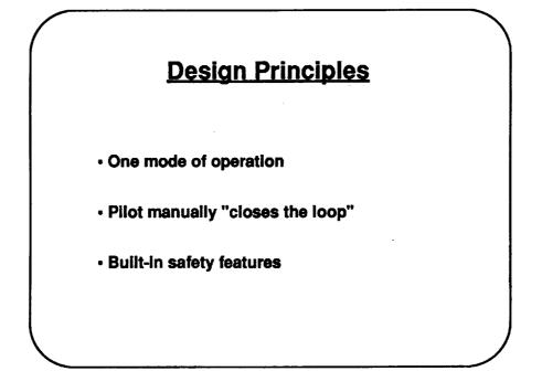
Although the simulated systems continually evolved as the tests were conducted, the evolution was guided by the principle that the there would be only one mode of operation for the entire maneuver. It was believed that having multiple modes of operations would ultimately lead to "mode errors" in which the pilot would forget which mode he was operating in and make an inappropriate input. Such mode errors have proved to be catastrophic in other highly automated airplanes.
