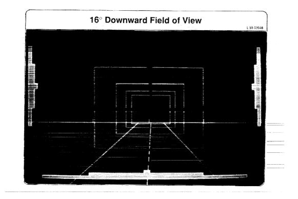
This picture was taken for same identical conditions as the previous slide except that downward field of view has been increased by 5° to 16°. The lane stripes are much more evident. The lane stripes can be aligned with the reference guide especially in the turns.
