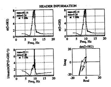
This slide is an example of the plot output from the CPE Analysis package. This is an actual plot of results that could be seen in the tunnel control room within about a minute from the completing the required data acquisition and could then be printed on a laserprinter in the control room. This data was used to aid in determining if we would go to the next test condition.
