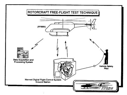
SLIDE 5: This slide depicts the test technique we are using to evaluate rotorcraft aerodynamics with FFRRV. The pilot sits in a ground based cockpit but perceives to be in the model via telepresence. The vehicle safety pilot has overall authority to interrupt the control system and terminate any experiment.
