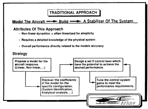
SLIDE 8: This is a "road map" to a traditional approach to developing a flight control system. These attributes are typical of model following control systems.
