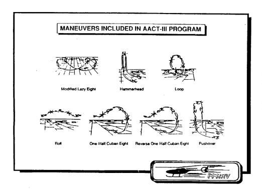
SLIDE 6: We want to look at aerodynamics in the "non-linear" world typical of air-to-air combat or nap-of-earth flying. This slide shows examples of maneuvering that characterize advanced combat rotorcraft. The researchers challenge is to quantify what makes a rotorcraft configuration more or less capable of such aggressive maneuvering.
