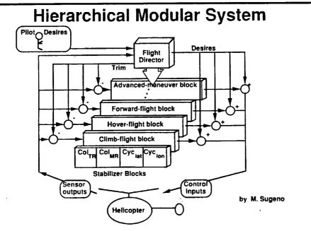
SLIDE 17: At first glance Professor Sugeno's controller appears like a simple gain scheduling controller. There are some significant differences: First, the lower level blocks are autonomous fuzzy logic controllers that can only perform their select mission. Secondly, the "gain scheduler" is not simply a mode switcher but is another fuzzy logic engine which blends the lower level blocks together to achieve a more abstract desire described by the pilot.
