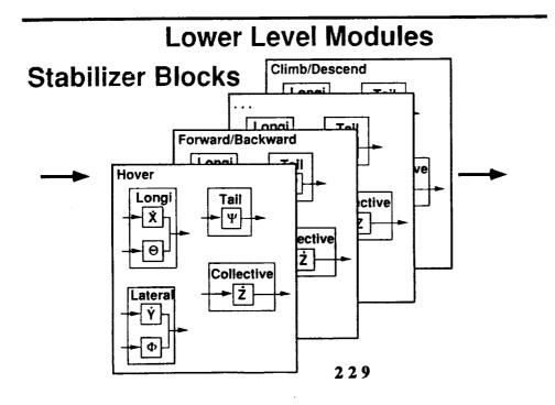
SLIDE 18: All the lower level stabilizer blocks have similar structure but each one is a unique multi-input/multi-output closed loop controller. The rule base and the fuzzy variable sets are different for each of these lower level blocks.
