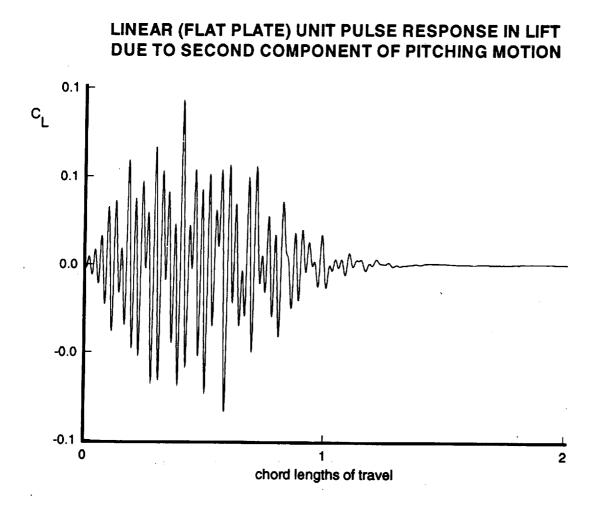
Linear (flat plate) Unit Pulse Response in Lift Due to Second Component of Pitching Motion
