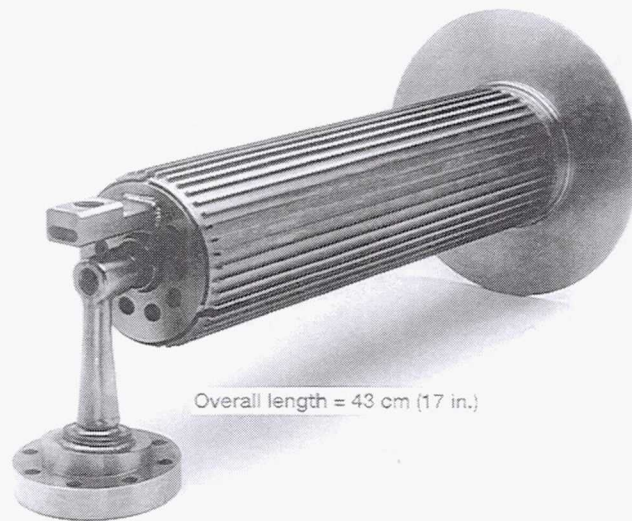
Figure 5.—Combustor liner, swirl plate, and fuel nozzle assembly.
