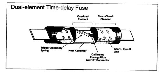
• Provide protection against low-level overload current or a short circuit current.
