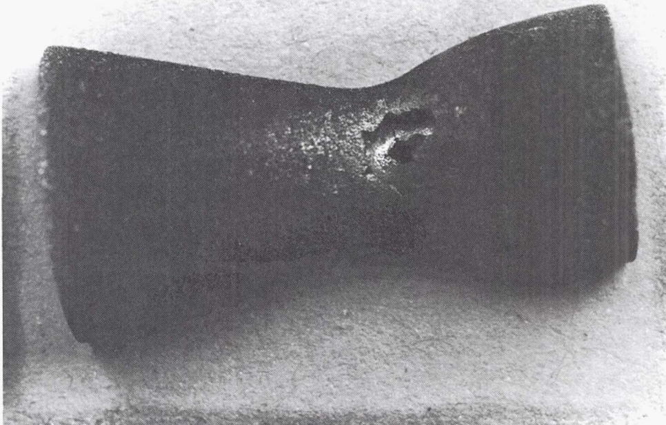
Figure 6.—Chamber 6063-1-10 (iridium-oxide composite coating) throat region exterior.
