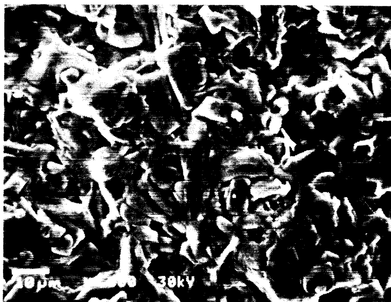
Figure 28. SEM micrograph of the grain structure of slip cast \text{YBa}_2\text{Cu}_3\text{O}_{7-x} .
