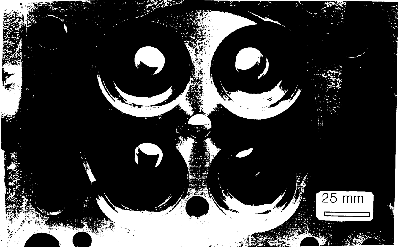
Figure 4.5: V903 cylinder head machined to accept a thermal barrier coating.
