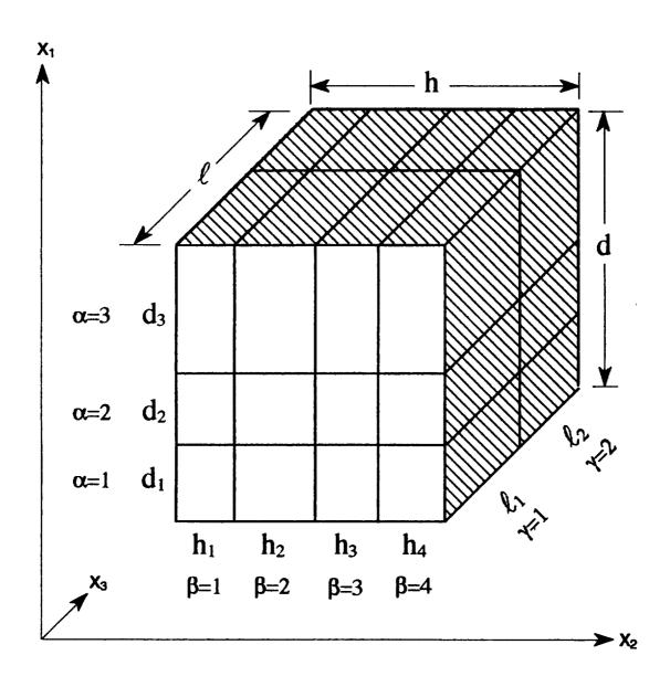
Fig. 1. (a) A repeating volume element that consists of  $N_{\alpha}=3, N_{\beta}=4$  and  $N_{\gamma}=2$  subcells.
