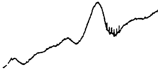
Figure 11. 35-GHz EPR spectra of SiO 2 rear or solar-facing exposure.
