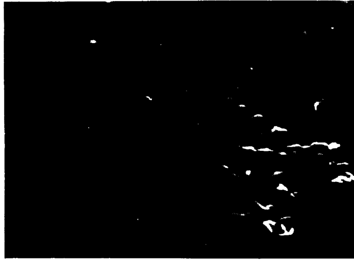
Figure 5. SEM study of crystal growth figures on a polyimide surface after flight on MIR.
