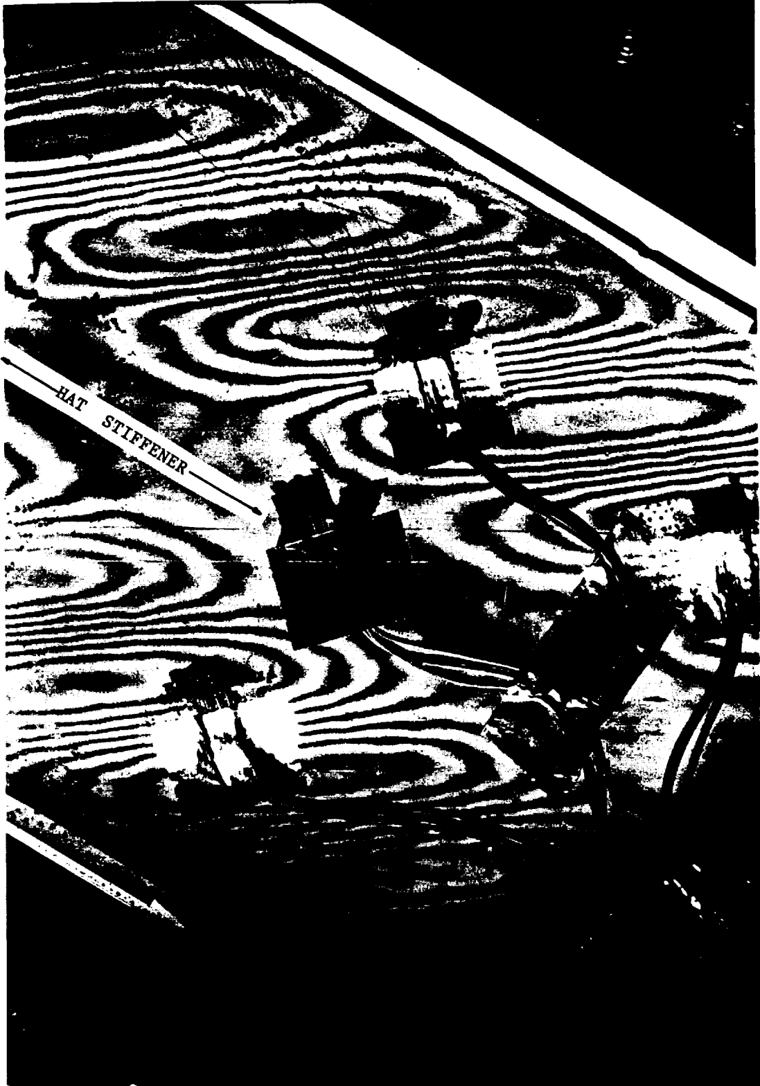
FIGURE 4.26. SHADOW MOIRE FRINGES NEAR FAILURE OF FRAME-STIFFENER INTERSECTION SPECIMEN (20000 LBS)
