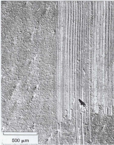
Figure 5.—Optical micrograph of soft 440C steel surface after rubbing with a 440C bearing ball. Lubricant: 50Å Fomblin Z-25.
