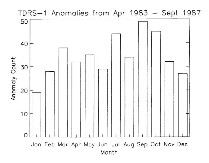
Figure 6. Graph made from data in anomaly database of anomalies on TDRS-1 weekly count for all observed SEU's. The rate shown is a minimum. The spikes in August, September and October are due to flares. (Source NGDC)
