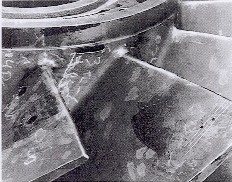
Figure 5.—Ports machined into the blade trailing edges for instrumentation.
