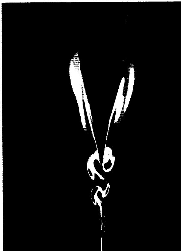
Figure 5-8. Vortex Flow Patterns of Edge Tone Stages
