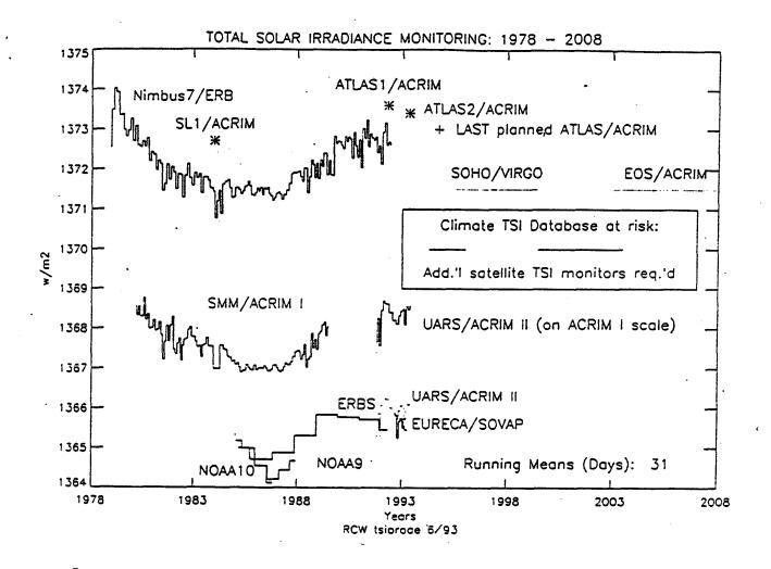
Figure 1. Measured total solar irradiance from 1978 through 2009 showing 31-day running mean measurements taken from orbit and planned future mission launch dates. (From Willson, 1993).
