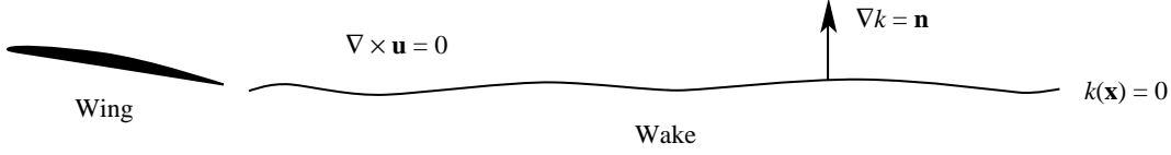
Figure 7. Thin wing in incompressible, irrotational flow with wake.
