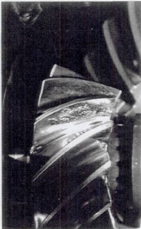
Figure 3.—Photograph of pinion damage at t = 8.55 hr.
