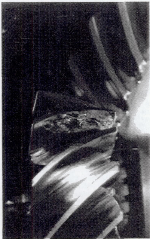
Figure 4.—Photograph of pinion damage at t = 10.03 hr.
