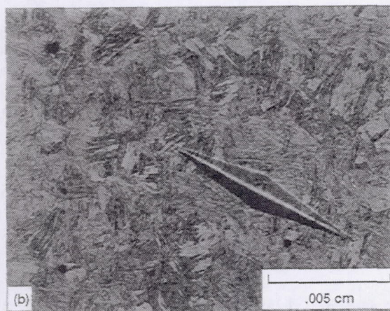
Figure 2.—Photomicrographs of case and core of CVM AISI 9310 spur gears. (a) Case. (b) Core.
