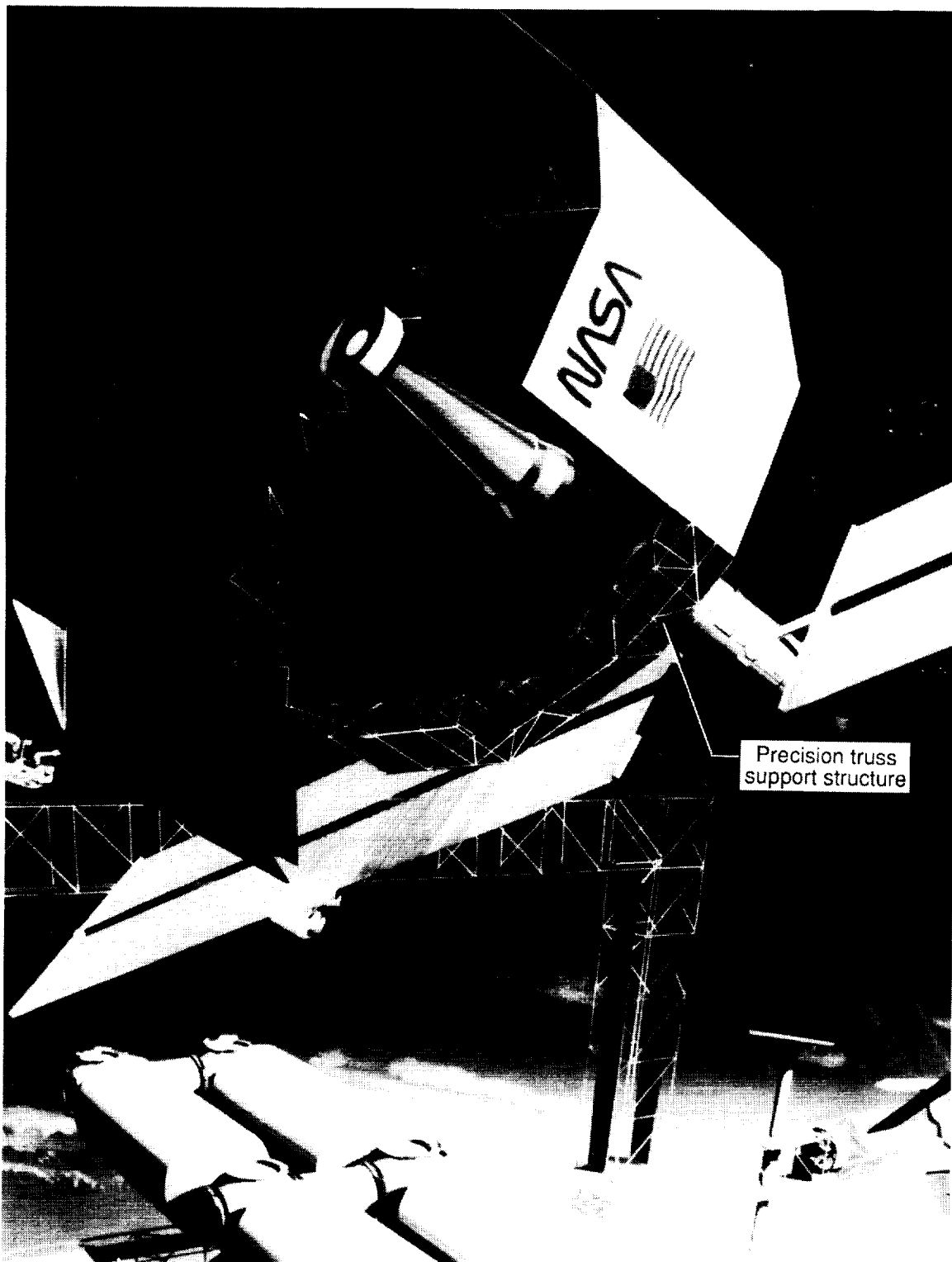
Figure 1. Proposed submillimeter astronomical space telescope that incorporates a large precision truss-supported reflector.
