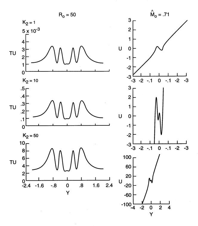
9. Vertical cuts at the vortex center of temperature perturbation due to the spanwise vorticity (TU) and streamwise velocity (U), for varying shear strengths. (No chemistry) Re = 50,  $M_0 = 0.71$ .
