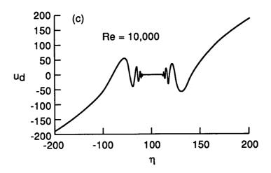
3. Plot of the solution difference  $u_d$  versus  $\eta$  for  $\Theta = \pm \pi/2$  and various values of the Reynolds number Re.
