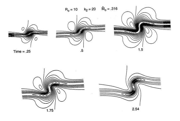
12. Contours of the temperature perturbation  $(T_1)$  evolution from early time to ignition. Re = 10,  $M_0 = 0.316, k_2 = 20$ .
