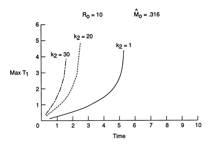
13. Plot of the maximum temperature perturbation  $(T_1)$  versus time for various shear strengths. Re = 10,  $M_0 = 0.316$ .
