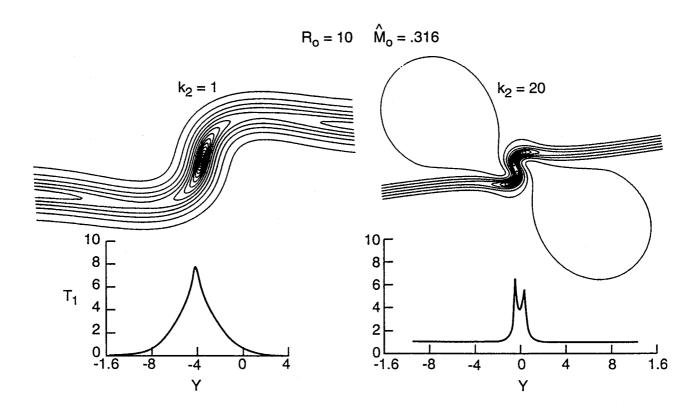
11. Contours and vertical cuts of the temperature perturbation  $(T_1)$  at ignition for increasing values of shear. Re = 10,  $M_0 = 0.316$ .
