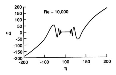
5. Plot of the solution difference  $u_d$  versus  $\eta$  for  $\Theta=\pm\pi/2$  and Re = 10,000.
