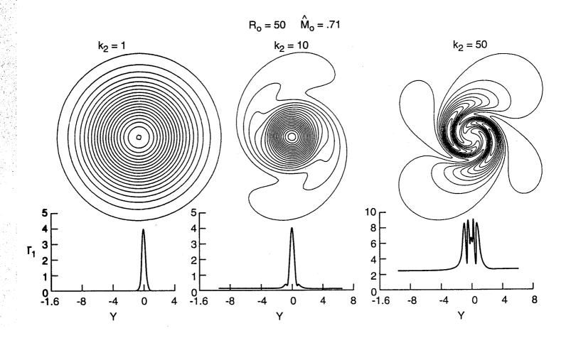
10. Contours and vertical cuts at the vortex center of the temperature perturbation  $(T_1)$  for increasing shear strengths. (No chemistry)  $T_1 = 50, M_0 = 0.71$ .
