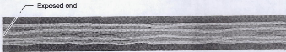
Figure 3.—T-3 specimen air aged for 500 hours at 316°C with 2% weight loss.
