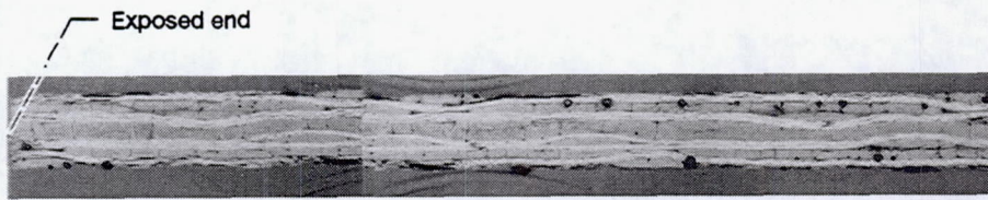
Figure 6.—T-3 specimen air aged for 1510 hours at 316°C with 10% weight loss.
