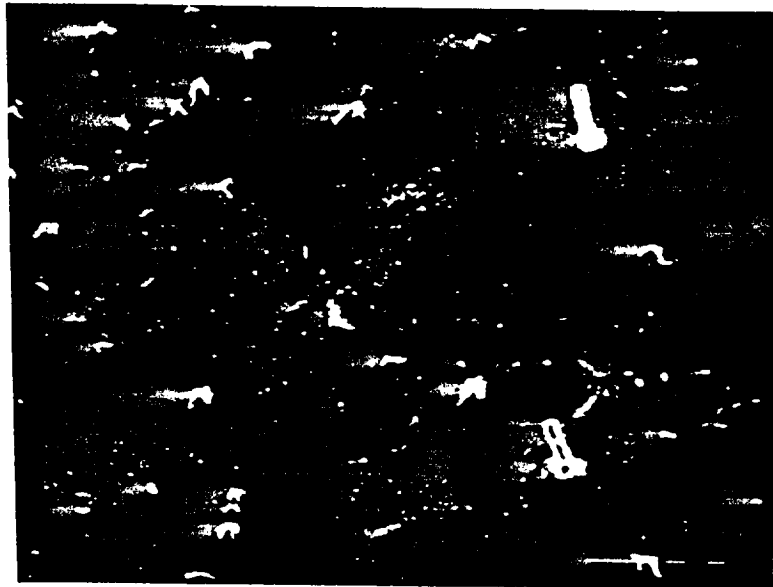
Figure 3. Scanning electron micrograph of decanted interface of MnBi-Bi solidifying at 2.98 cm/hr [31]. SEM magnification 3200 X. Average rod spacing \lambda approximately 4 \mu\text{m} .
