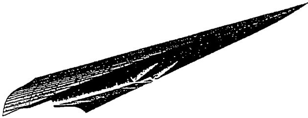
Fig. 1 Hypersonic vehicle concept with an integrated hydrocarbon scramjet engine.
