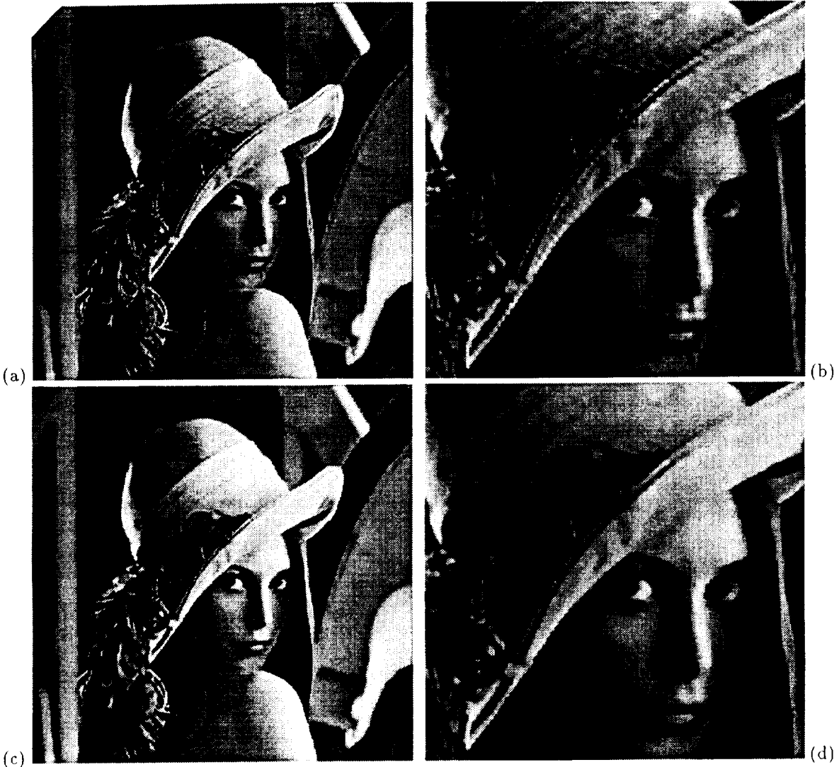
Fig. 7. VQ subband images (0.444 bpp): (a) standard decompression (b) enlarged (c) after 9-th iteration of postprocessing algorithm, T = 1.0 (d) enlarged.
