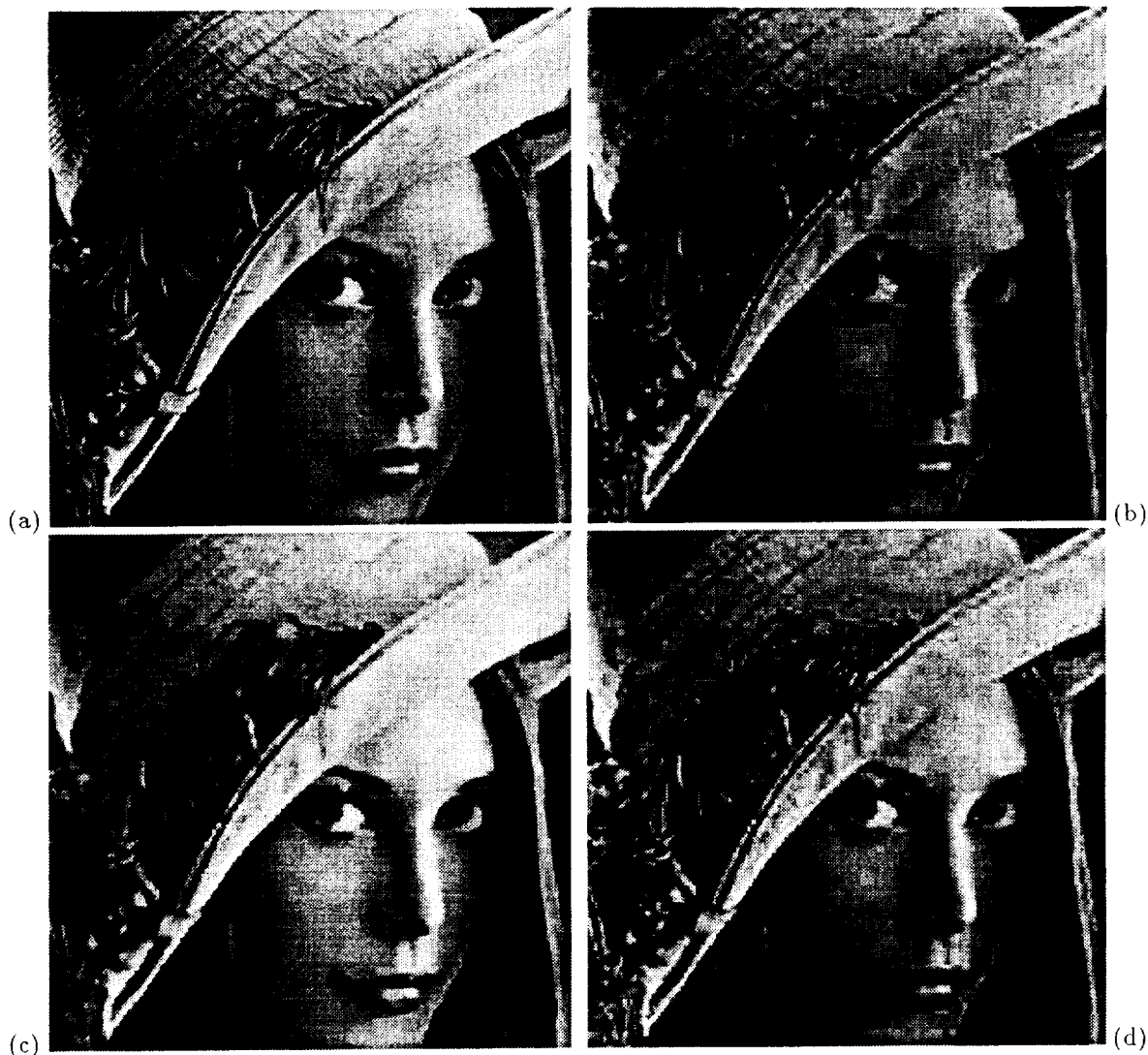
Fig. 5. Scalar quantization DCT compressed images (0.264 bpp) (enlarged view): (a) original image (b) standard decomposition (c) After 9-th iteration of postprocessing algorithm, T = 1.0 (d) reconstructed with AC coefficient prediction.
