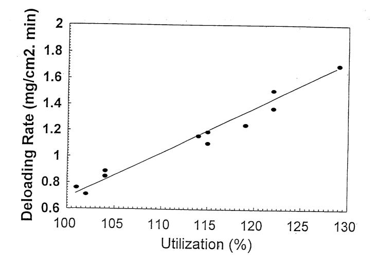
Figure 5. Correlation Between Deloading Rates and Utilization
