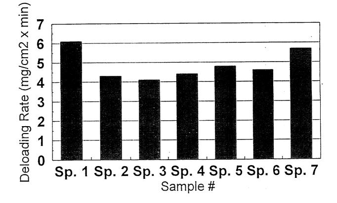
Figure 4. Deloading Experiment for Cadmium Plates, Lot 1B
