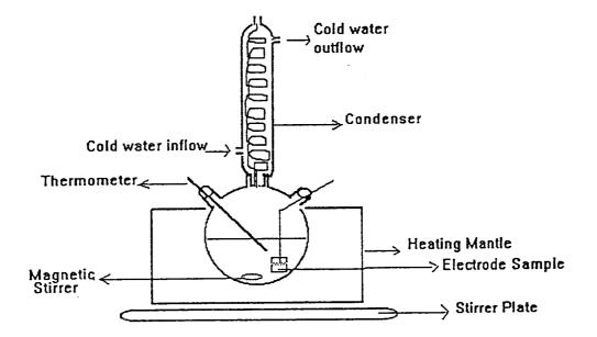
Figure 1. Schematic of the Deloading Experimental Setup
