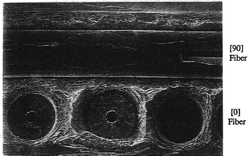
IP,  $S_{max} = 500$  MPa,  $N_f = 1\ 089$  100  $\mu\text{m}$
