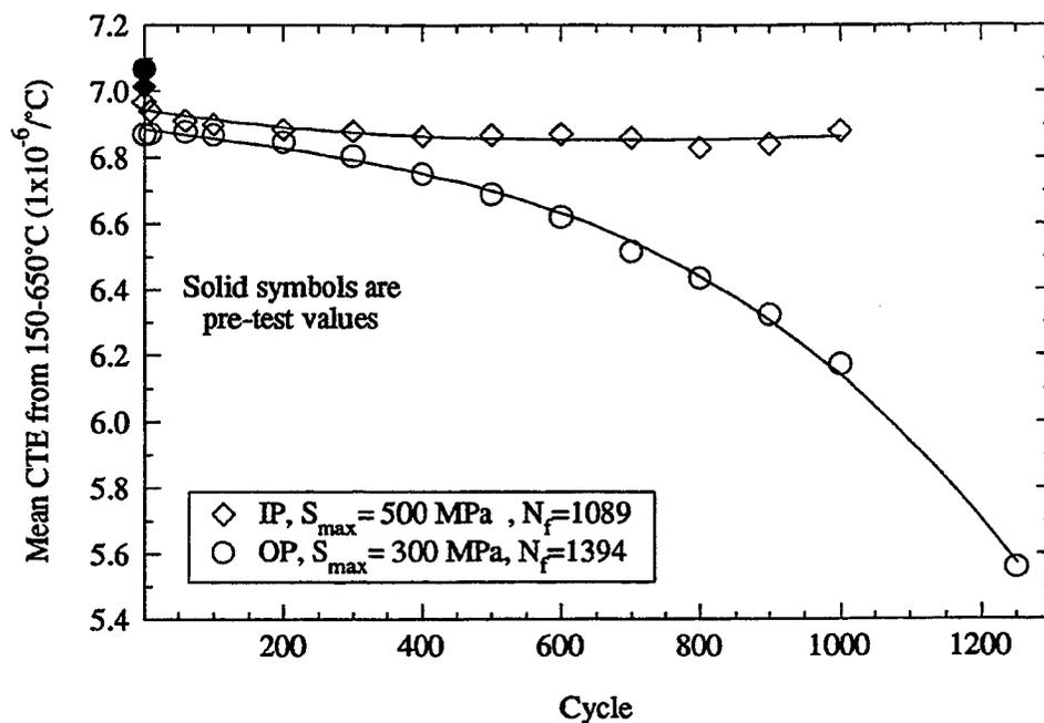
Figure 11. Degradation of the mean coefficient of thermal expansion from 150 to 650°C during IP and OP TMF of SCS-6/Timetal 21S [0/90]<sub>s</sub>.
