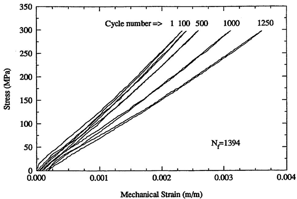
Figure 4. Out-of-phase thermomechanical fatigue deformation of SCS-6/Timetal 21S [0/90]<sub>s</sub> with  $S_{max} = 300$  MPa.
