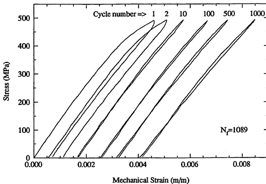
Figure 3. In-phase thermomechanical fatigue deformation of SCS-6/Timetal 21S [0/90]<sub>s</sub> with  $S_{max} = 500$  MPa.
