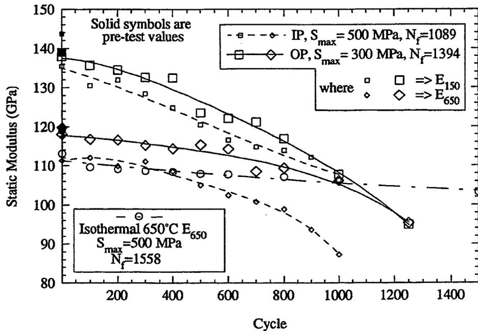
Figure 10. Degradation of the isothermal static moduli at 150 and 650°C during IP and OP thermomechanical fatigue of SCS-6/Timetal 21S [0/90]<sub>s</sub>.
