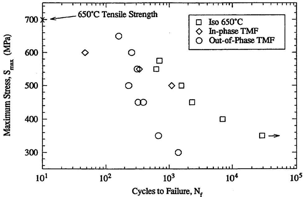
Figure 2. Thermomechanical fatigue life of SCS-6/Timetal 21S [0/90]<sub>s</sub> with a temperature cycle of 150-650°C.
