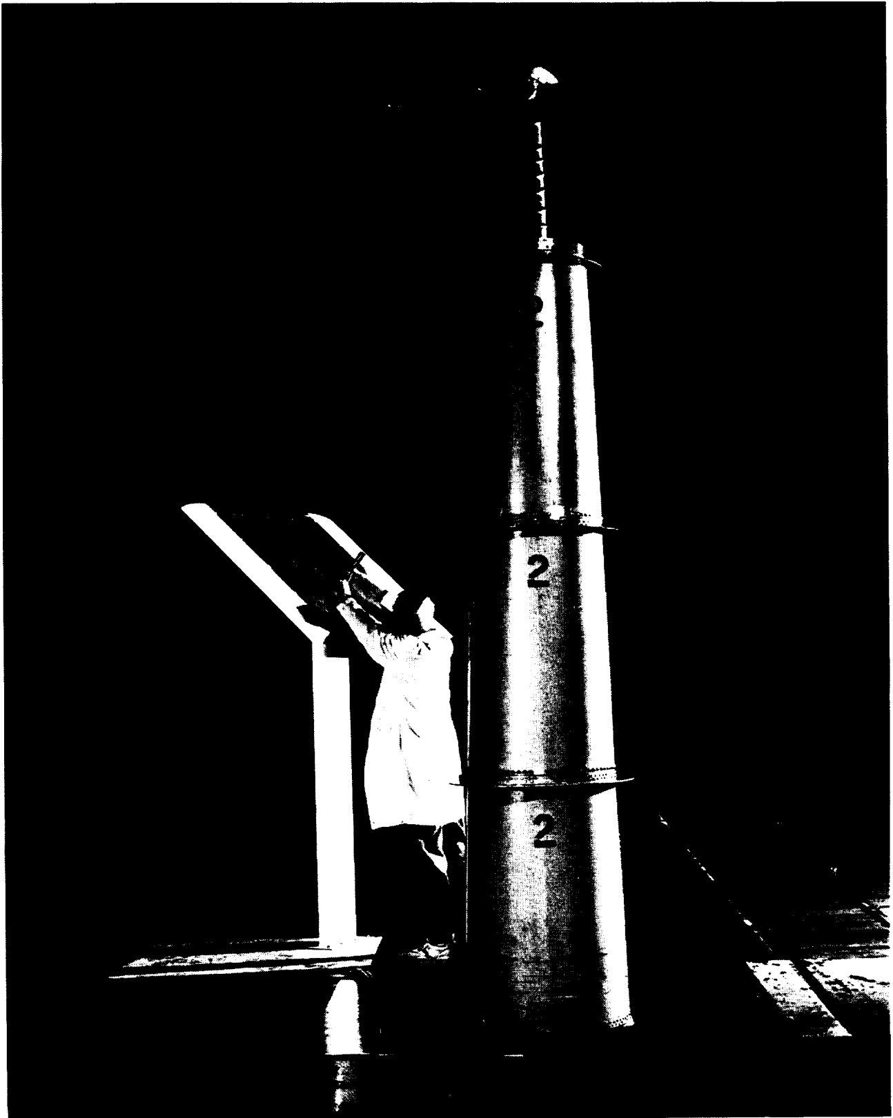
Figure 28. Phased microphone array being calibrated in the 40 × 80.
