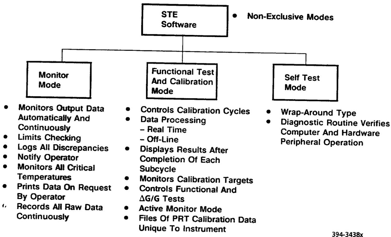
Figure 11 The Special Test Equipment Software Characteristics and Functions
