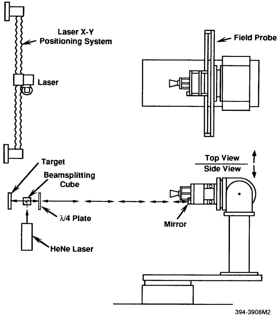
Figure 25 Compact Range Laser Alignment System
