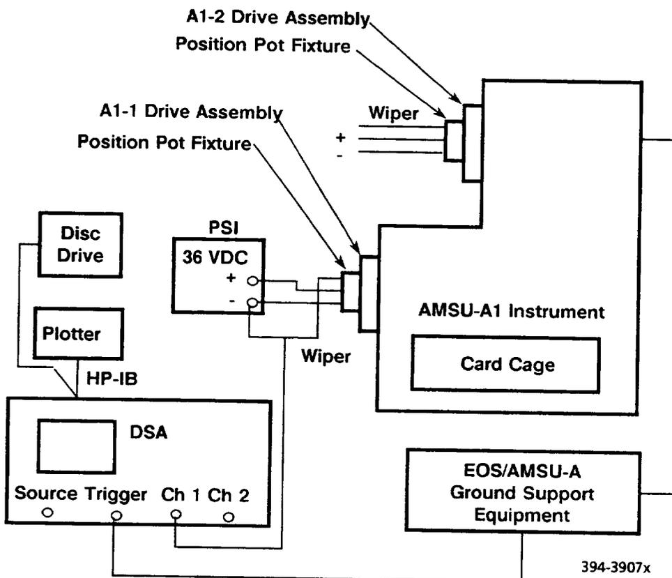
Figure 26 Test Setup for Antenna Position Measurement
