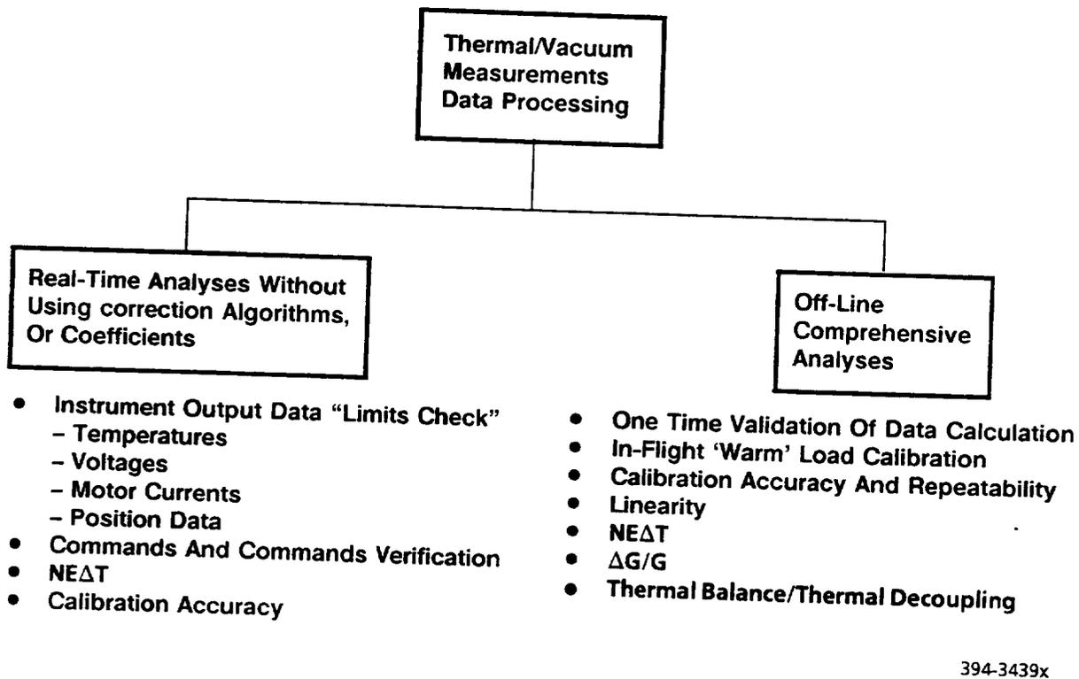
Figure 18 Thermal Vacuum Measurements Data Processing
