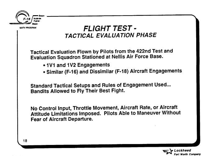
For the MATV program, a new control law was developed using multi-axis thrust vectoring to augment the aircraft's aerodynamic control power to provide maneuverability above the normal F-16 AOA limit. The control law architecture was developed using Lockheed Fort Worth's offline and piloted simulation capabilities. The final flight control laws were used in flight test to demonstrate tactical benefits gained by using thrust vectoring in air-to-air combat.
