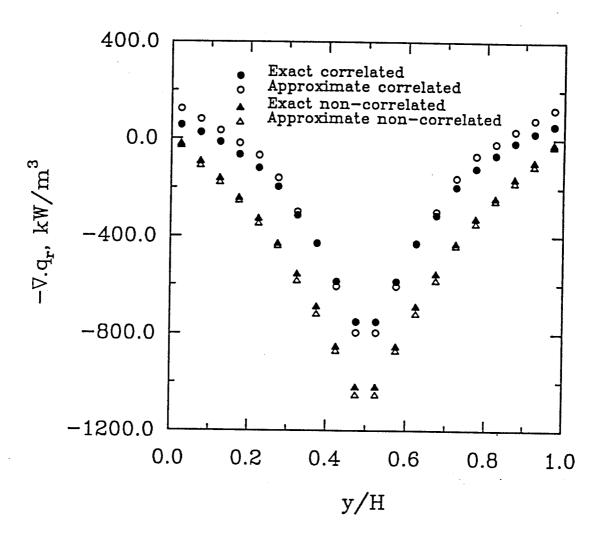
Fig. 5.8 Radiative source distribution at the location x/L=0.825 for nonisothermal and inhomogeneous  $H_2O-O_2-N_2$  mixture.
