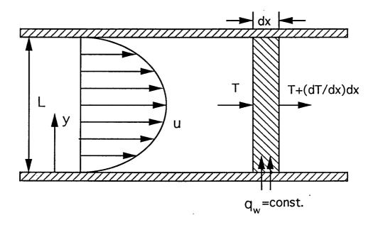
Fig. 4.1 Laminar flow between parallel plates with constant wall heat flux.
