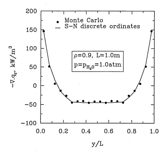
Fig. 3.11 Comparison of radiative source term in pure  $H_2O$  for  $\rho=0.9$ , L=1.0 m.
