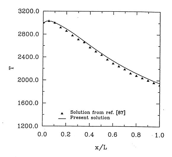
Fig. 6.6 Comparison of reacting temperatures along the centerline.
