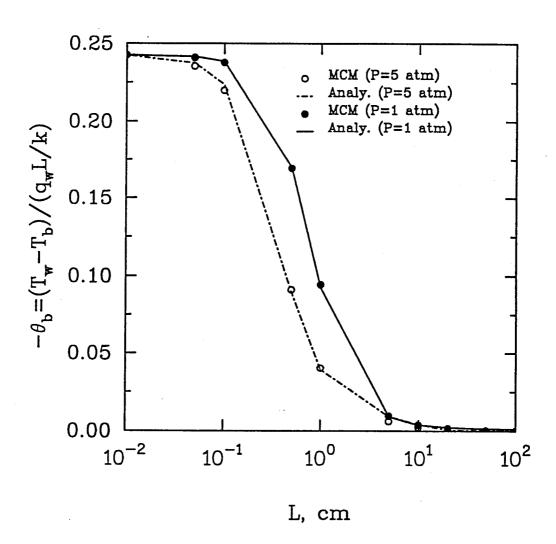
Fig. 4.3 Comparison of gray solutions for  $CO_2$  at  $T_w$ =1000 K.
