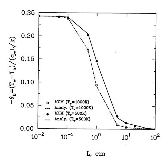
Fig. 4.2 Comparison of gray solutions for  $CO_2$  at p=1 atm.
