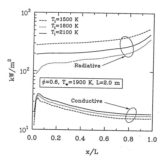
Fig. 6.18 Comparison of radiative and conductive wall fluxes for three different inlet temperatures.
