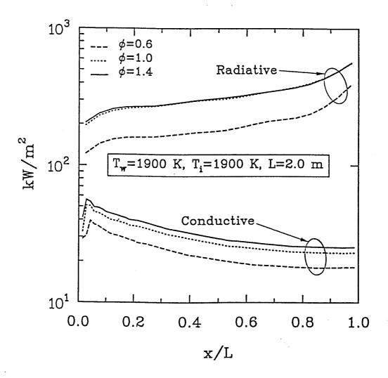
Fig. 6.16 Comparison of radiative and conductive wall fluxes for three different equivalence ratios.
