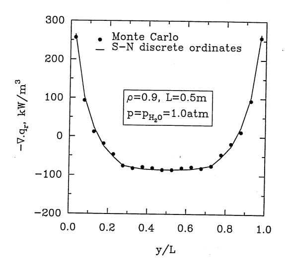
Fig. 3.9 Comparison of radiative source term in pure  $H_2O$  for  $\rho$ =0.9, L=0.5 m.
