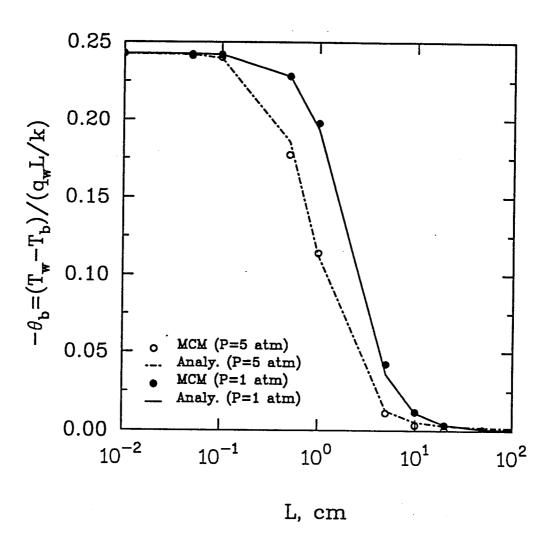
Fig. 4.5 Comparison of gray solutions for  $H_2O$  at  $T_w$ =1000 K.
