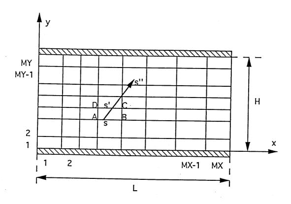
Fig. 5.1 Schematic of two finite parallel plates and grid configuration.
