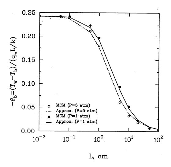
Fig. 4.7 Comparison of nongray solutions for  $CO_2$  at  $T_w$ =1000 K.
