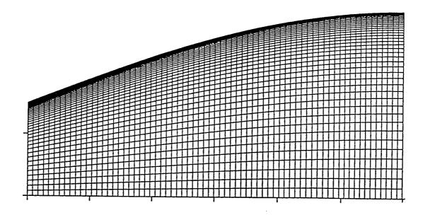
Fig. 6.2 Grid mesh for flowfield simulation.
