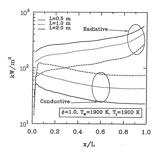
Fig. 6.19 Comparison of radiative and conductive wall fluxes for three different nozzle sizes.
