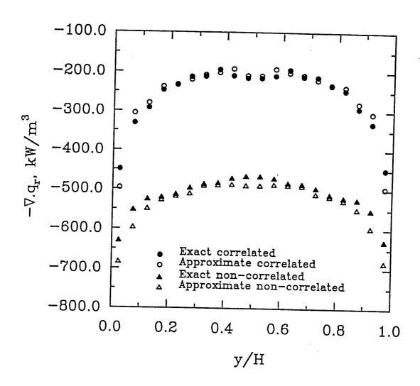
Fig. 5.4 Radiative source distribution at the location x/L=0.5 for isothermal and homogeneous  $H_2O-N_2$  mixture.
