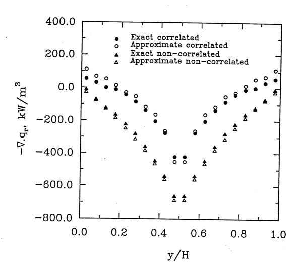
Fig. 5.7 Radiative source distribution at the location x/L=0.5 for nonisothermal and inhomogeneous  $H_2O-O_2-N_2$  mixture.
