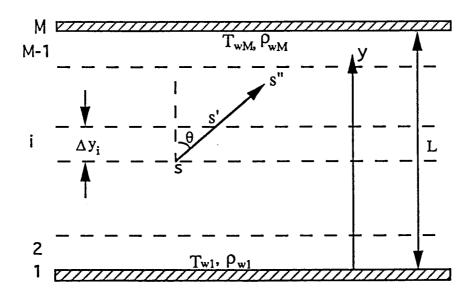
Fig. 3.1 Planar medium between two parallel walls.
