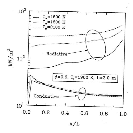
Fig. 6.17 Comparison of radiative and conductive wall fluxes for three different wall temperatures.
