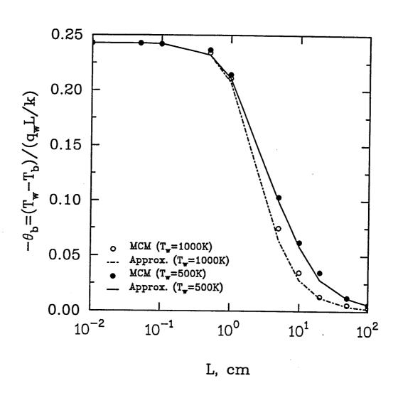
Fig. 4.8 Comparison of nongray solutions for H<sub>2</sub>O at p=1 atm.
