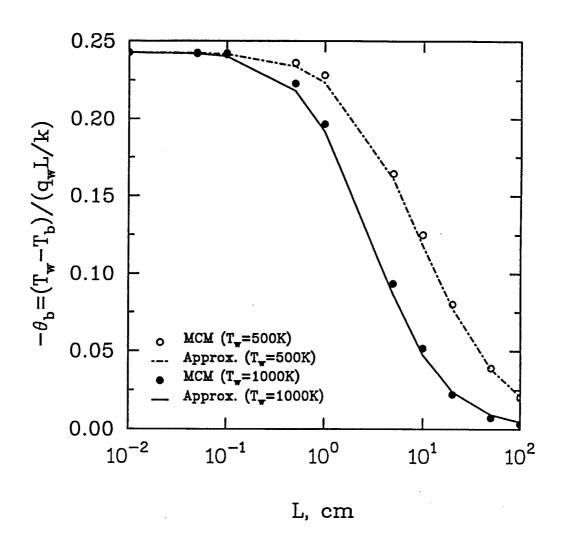
Fig. 4.6 Comparison of nongray solutions for  $CO_2$  at p=1 atm.
