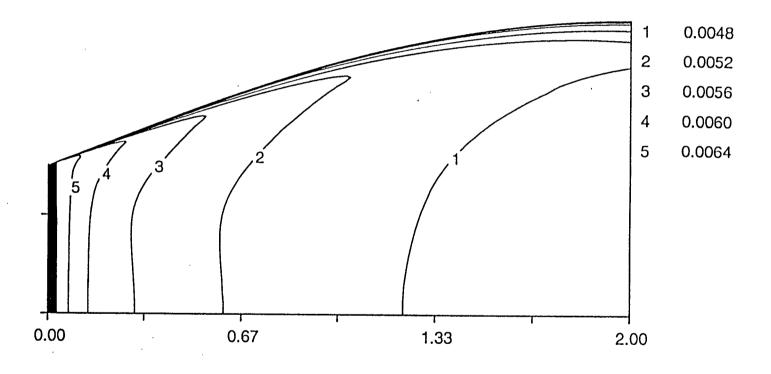
Fig. 6.13 H<sub>2</sub> mass fraction contours in the nozzle.
