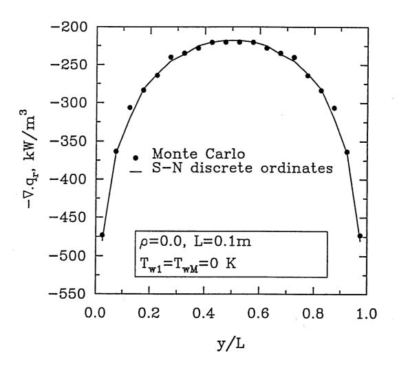
Fig. 3.3 Comparison of radiative source term for the uniform temperature profile with L=0.1 m.
