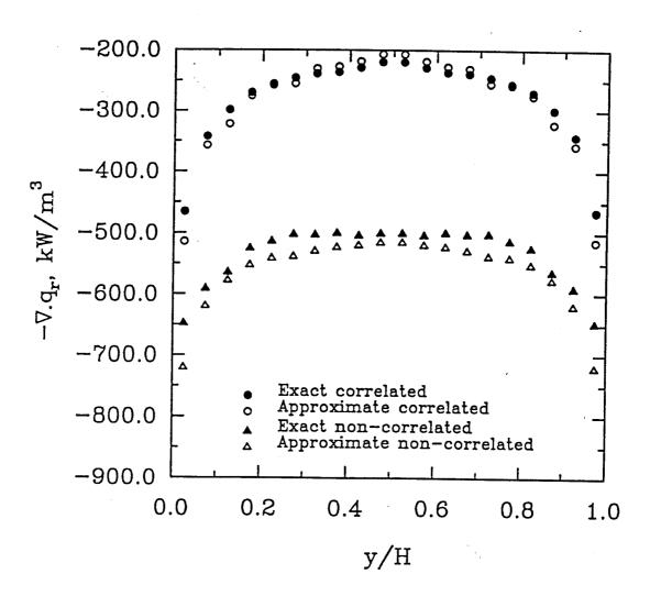
Fig. 5.3 Radiative source distribution at the location x/L=0.225 for isothermal and homogeneous  $H_2O-N_2$  mixture.
