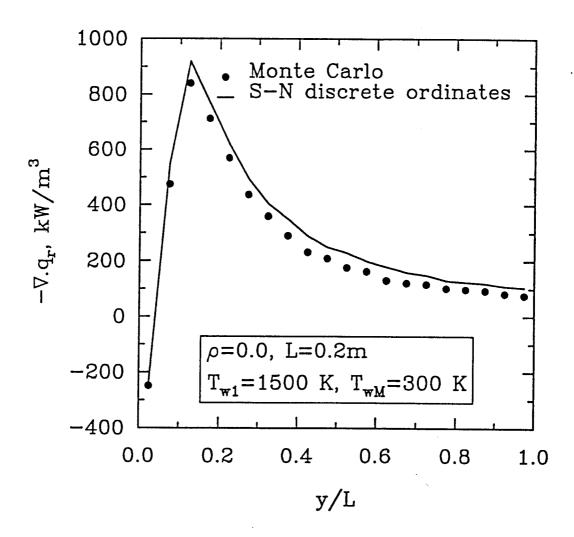
Fig. 3.5 Comparison of radiative source term for the boundary layer type temperature profile.
