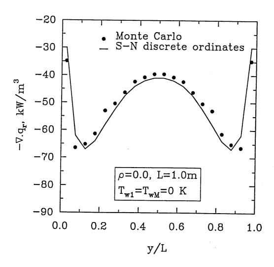
Fig. 3.6 Comparison of radiative source term for the parabolic H<sub>2</sub>O concentration profile.
