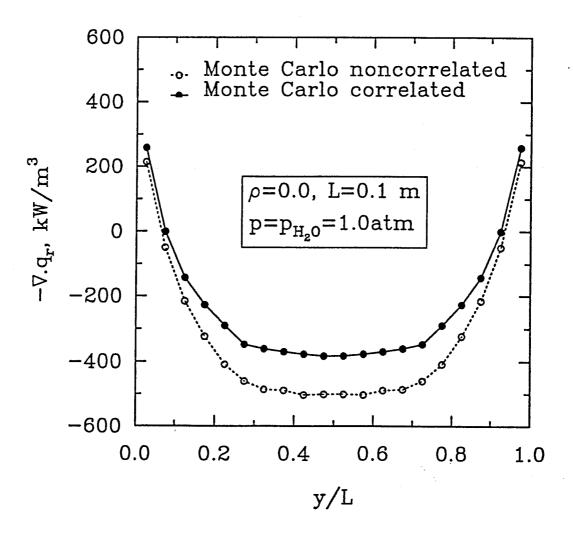
Fig. 3.12 Comparison of correlated and noncorrelated results in pure  $H_2O$  for  $\rho$ =0.0, L=0.1 m.
