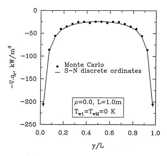
Fig. 3.4 Comparison of radiative source term for the uniform temperature profile with L=1.0 m.
