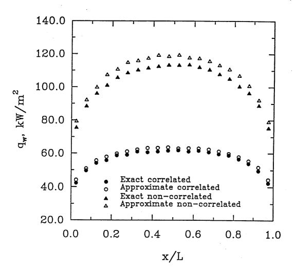
Fig. 5.5 Radiative wall flux distribution for isothermal and homogeneous H<sub>2</sub>O-N<sub>2</sub> mixture.
