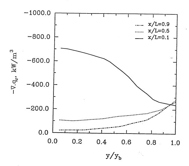
Fig. 6.15 Radiative source distribution at three locations.
