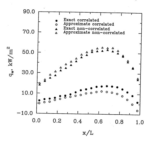
Fig. 5.9 Radiative wall flux distribution for nonisothermal and inhomogeneous  $H_2O\!-\!O_2\!-\!N_2$  mixture.
