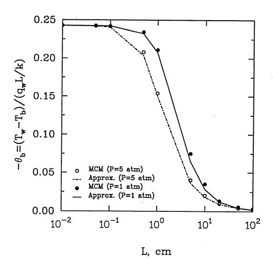
Fig. 4.9 Comparison of nongray solutions for H<sub>2</sub>O at T<sub>w</sub>=1000 K.
