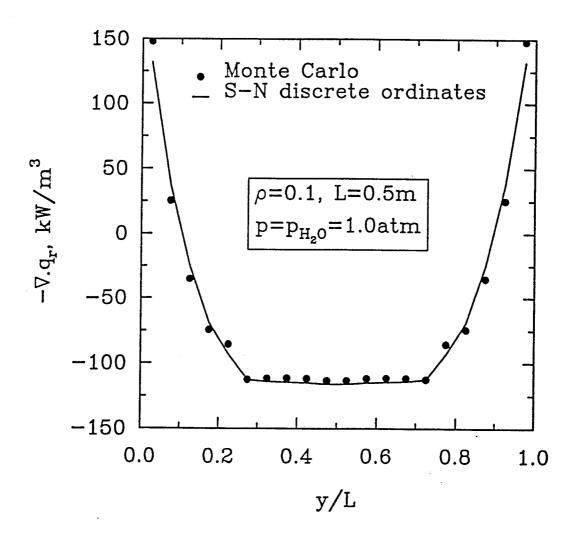
Fig. 3.7 Comparison of radiative source term in pure  $H_2O$  for  $\rho$ =0.1, L=0.5 m.
