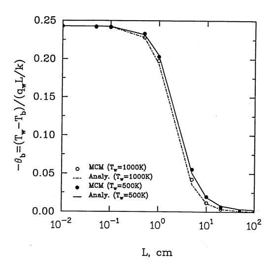
Fig. 4.4 Comparison of gray solutions for H<sub>2</sub>O at p=1 atm.
