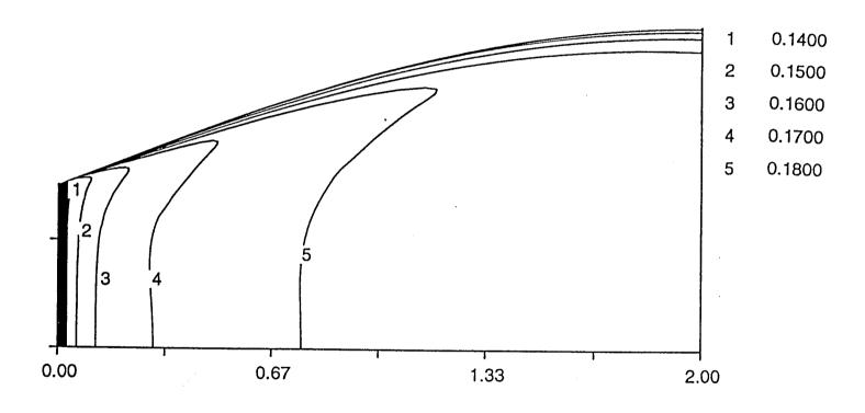
Fig. 6.11 H<sub>2</sub>O mass fraction contours in the nozzle.
