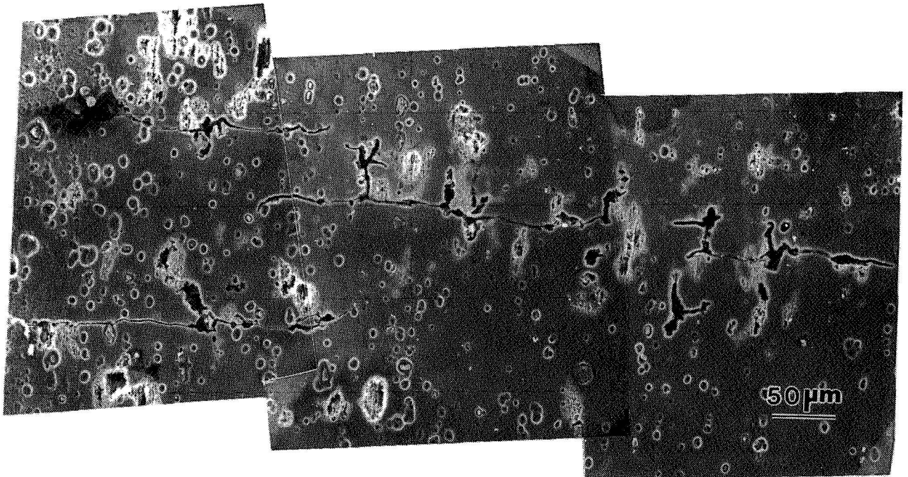
Figure 11. Secondary cracks forming (away from the main crack) at corrosion pits at the free surface of a fatigue specimen tested in 0.5M NaCl solution at room temperature with \sigma_{\max} = 320 MPa ( R = 0.1 ) and with f = 0.1 Hz.
