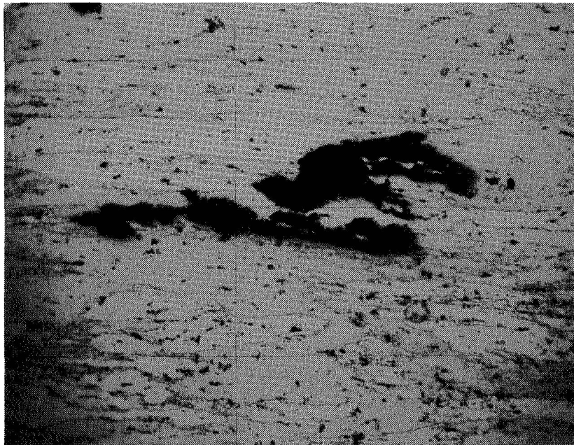
Fig. 8. Corrosion pits on the exposed surface of the specimen showing pit growth in the rolling direction, magnification 100X.
