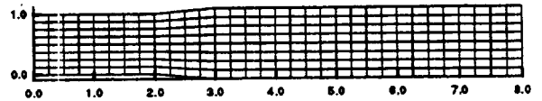
Figure 20 a. Computational grid for a diverging channel. Ramp angle = 5 degrees. 32 \times 8 grid.
