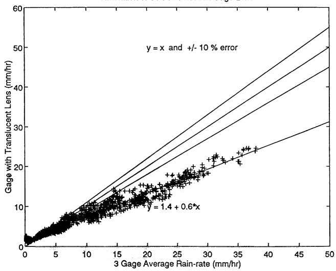
Simulation of Sea Salt on Rain Gage Lens
