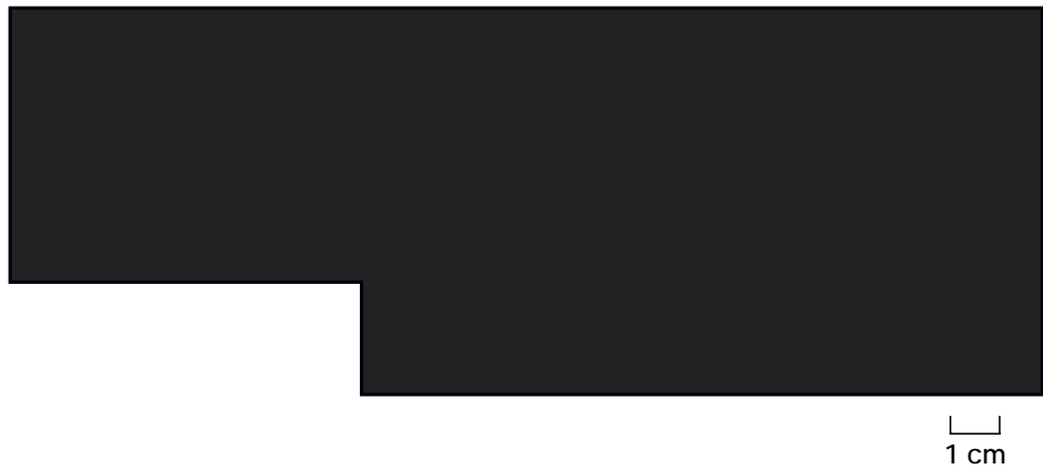
Figure 6.—Film radiography. Source-to-panel distance = 30 in., 60 kV, 25 mA, 2 min. Panel appears uniform. Indicates density variations below ~ 2% if thickness variations insignificant.
