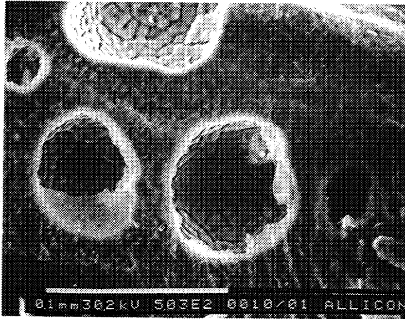
Figure 3. - Blisters on the free surface of a contaminated weld showing evidence of surface melting and gas pressure.
