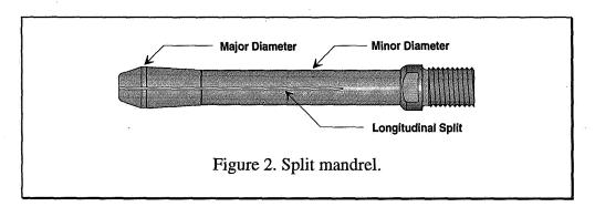
The only difference between the split mandrel (SpM) and split sleeve (SpSI) system for coldworking holes is the design of the tooling system utilized in performing the work. The split mandrel process
