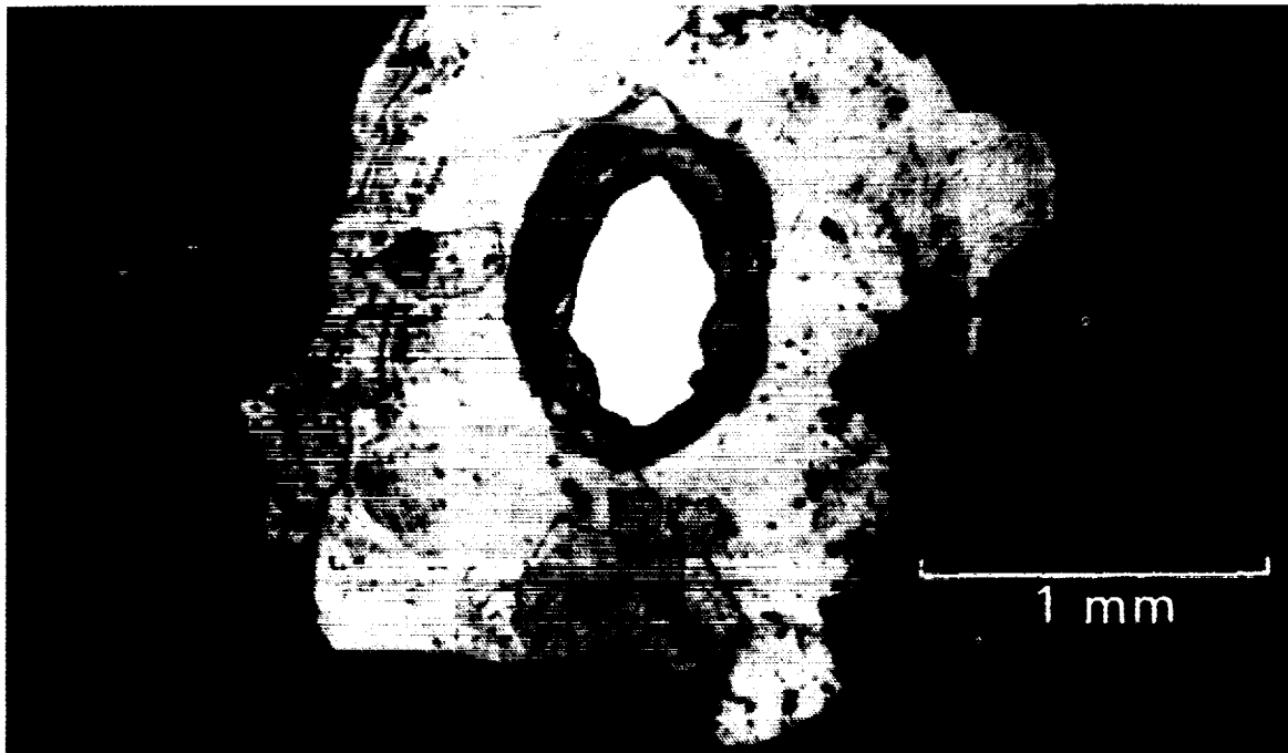
Figure 6. Evaporation of polymer and metal due to discharge in electron-irradiated aluminized Kapton. Magnification \times 12 (Verdin, 1980).
