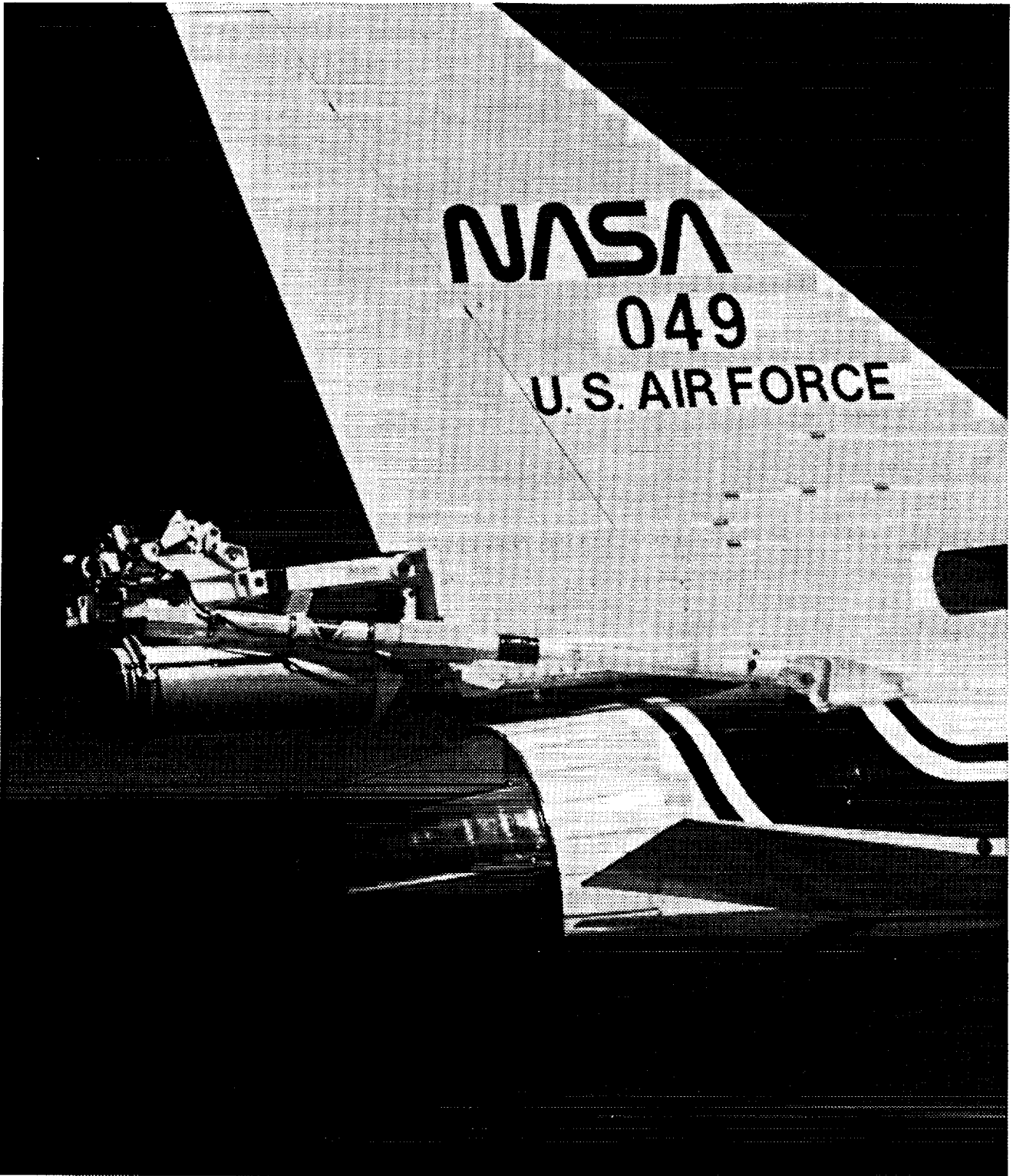
Figure 3. The X-29A no. 2 spin chute assembly.
