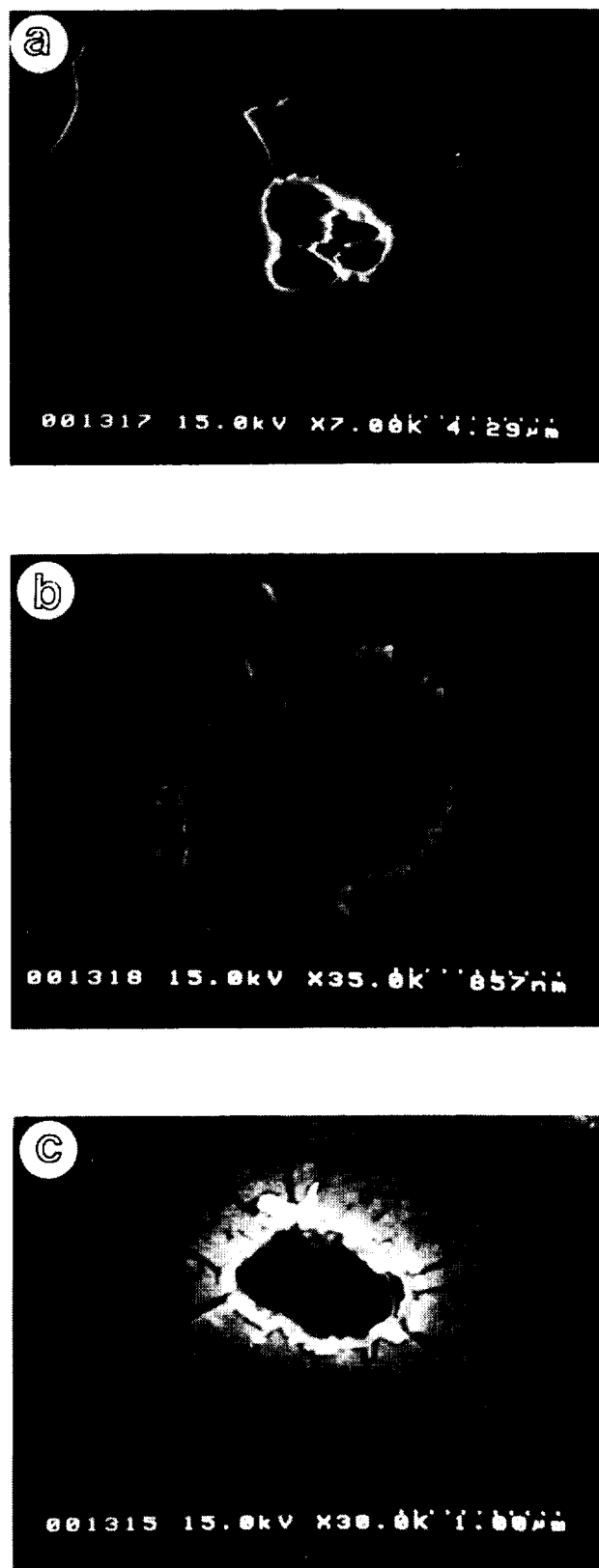
Fig. 10. SEM images of ZnS formed craters in glass: (a) 4.6 km sec -1 crater. Impactor apparently separated into 3 fragments at impact. Impactor size was 0.0089 mm. (b) 6.4 km sec -1 crater. Cracked surface is due to breakup of Au coating with time. Impactor dia. was 0.001 mm. (c) 10.1 km sec -1 crater. Impactor dia. was 0.00066 mm. All crater outlines depart from circularity. All launches were 90° to the target and all rims contain detectable Zn.
