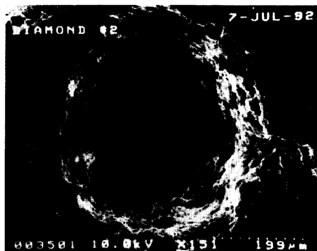
Fig. 4. Diamond crater made at 5.1 km sec -1 . Note the great depth and irregular cavity. Essentially no residual diamond; only PCG.
